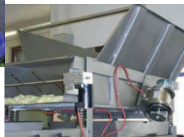
Conveying with stainless steel electric external vibrators
