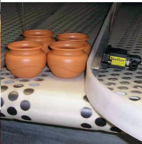
Loosing product compaction with pneumatic circular oscillators
