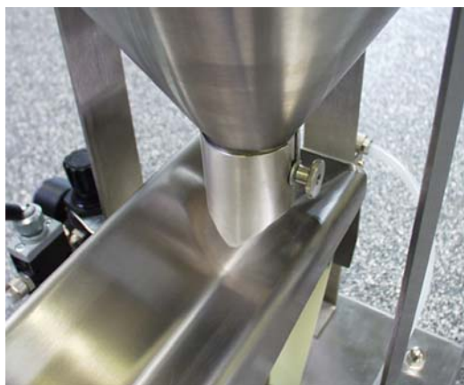
Dosing port at the silo outlet
