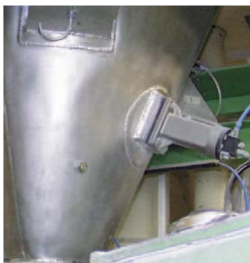
Cleaning bunker walls
